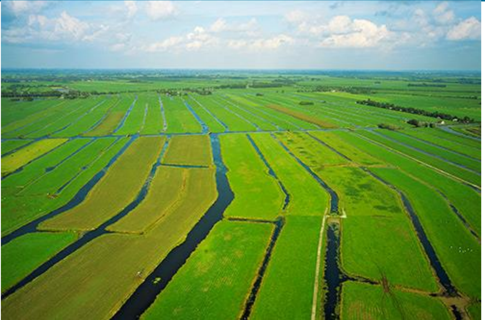
Reclamation of land and dewatering by digging ditches
